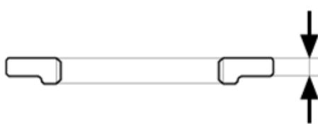
**止推垫圈,  $40 \times 63 \text{ mm}$**
